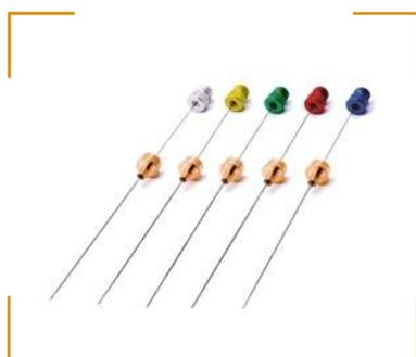
Solid phase microextraction-GC-MS (SPME-GC-MS)
