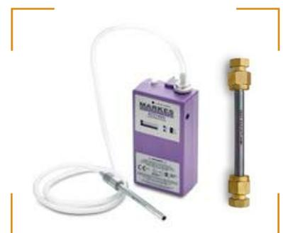
Cartridges fill-in with sorbent material for on-site sampling and TD-GC-MS analysis
